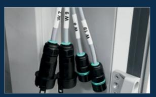
Prepared and encoded connectors for easy cabling.
